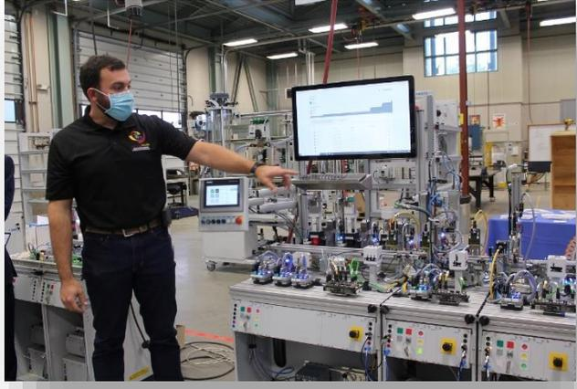
Of particular interest was a new lab of equipment to be used starting this spring by students in Hartnell's new Mechatronics Technician program. Called an "Industry 4.0 and Cyber Physical Systems Workshop," the equipment includes collaborative robots, mobile robots and smart sensors with io-Link and distributed io, all manufactured by FESTO Corp. These learning tools can be used to train students in such fields as hydraulic and pneumatic systems and machine learning/machine vision.
